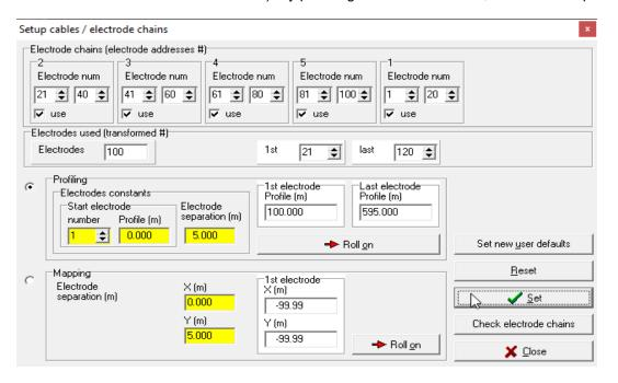
The 1<sup>st</sup> electrode now in use is the electrode number 21 (address 21) at position = 100 m. The last electrode in use is the number 120 (address 20) at position = 595 m. This setup is used for the next measurement. After the  $2^{nd}$  measurement, the resulting pseudosection looks like this:
