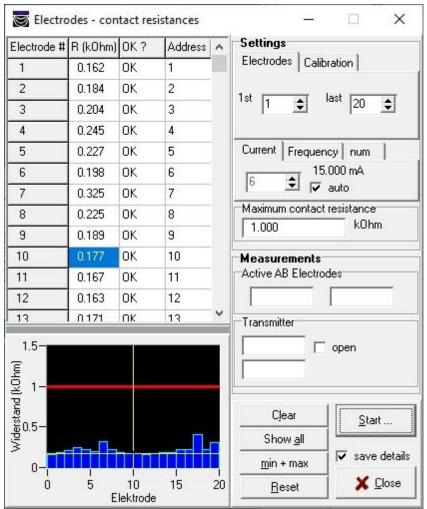
This form controls the measurement of **contact resistances**. The contact resistance is the resistance (= impedance, measured in Ohm =  $\Omega$ ) between one electrode and ground. Although the measurements are done by pairs of electrodes, the contact resistance of each measured electrode is calculated and shown against the respective electrode number. For comparison, the respective electrode address is shown too.
