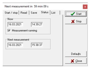
**Now:** The current date and time is displayed. The checkbox "Measurement running" is checked during the active measurement. It is unchecked during the waiting period.
