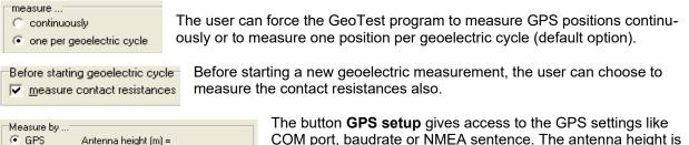
COM port, baudrate or NMEA sentence. The antenna height is the vertical distance between the GPS antenna and the ground.
