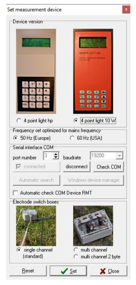
**Device version:** The hardware version "4 point light hp" (older version manufactured until 2007, grey case, left side) uses a fixed serial baudrate of 1200. The hardware version "4 point light 10W" (newer version manufactured since 2007, red and black case, right side) allows to choose a maximum serial baudrate up to 38400.
