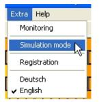
The simulation mode is used to test the sequence of electrode switchings and measurements. During running the simulation mode, all readings and settings are simulated and not really per formed. This may be a useful option to test complex measurement arrays.
