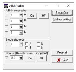
This form gives direct access to the active electrodes (ActEle). The user may switch a specific address to A,B,M,N function or off. A and B = power emitting current electrodes. M and N = voltage measuring potential electrodes.
