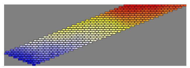
The data is saved. The example procedure is repeated again: roll-on + measure + save. After  $2^{nd}$  roll-on procedure (in total  $3^{rd}$  measurement), the total profile reaches now up to electrode number 140 = 695 m.
