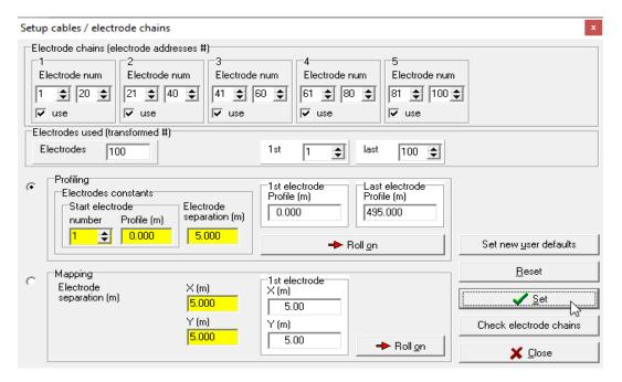
This setup shows in total 100 electrodes. The  $1^{st}$  electrode in use (address 1) is at profile start = 0 m. The last electrode number 100 (address 100) is situated at the profile end = 495 m. The user fixes this setup by pressing "Set", sets all profile settings (main menu > set > electrodes and data header) and starts the measurement (main menu > measure > start ...). After finishing the  $1^{st}$  measurement, the respective pseudosection of the example looks like this:
