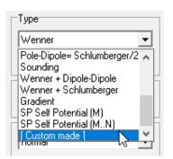
After choosing **[ Custom made ]** and pressing **Set** a new window appears. This window allows the setting of A, B, M and N electrode numbers by the user. This example shows some Schlumberger sounding with potential electrodes M=10 and N=11. The user has extended the sounding configurations by adding values for M=8 and N=13.
