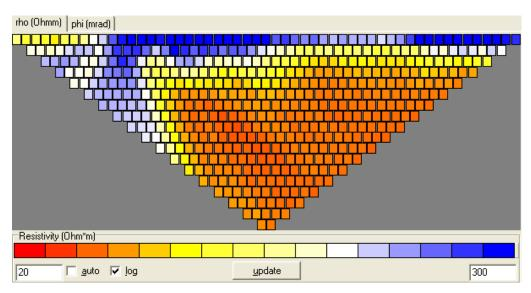
The pseudo section displays the measured data as colored boxes. The boxes are situated in some table type refering to the horizontal and vertical positions of the respective measurement. These sections are called "pseudo", because the vertical positions of the boxes are - of course - not the real vertical positions of the respective data point. For getting quasi real vertical positions, some evaluation of data is necessary (computer inversion modelling).
